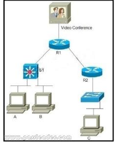
For multicast traffic, where must the filtering be placed to fulfill that requirement? A. R1 B. Video Conference C. A D. S1 E. R2 Answer: D QUESTION 87 Which two VPN solutions extend the routing capabilities of basic IPsec VPNs? (Choose two.)
