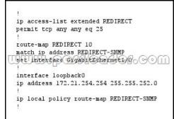
A. All SNMP traffic coming into the router is redirected to interface GigabitEthernet1/0.
