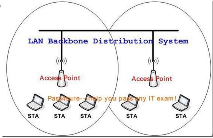
A:Access points in each cell must be configured to use channel 1. B:The network diagram represents an extended service set (ESS). C:The area of overlap of the two cells represents a basic service set (BSS). D:The area of overlap must be less than 10% of the area to ensure connectivity. E:The two APs should be configured to operate on different channels. **Correct Answers: B, E**
