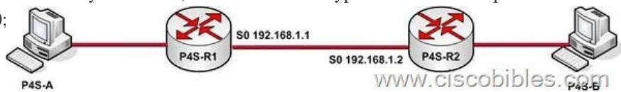
**Lab Requirements:** Configure the routers with RIP version 2(RIP-2)so that all devices can ping any other device. **Lab Process:**
