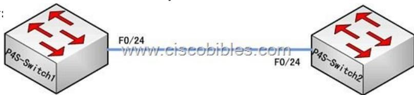
**Lab Requirements:** 1. Port F0/24 of SW1 is connected with Port F0/24 of SW2. Set the two ports to trunk mode. 2. Set SW1 to VTP server mode and SW2 to VTP client mode. 3. SW1 creates VLAN2. Check whether VLAN information can be synchronized on SW2.
