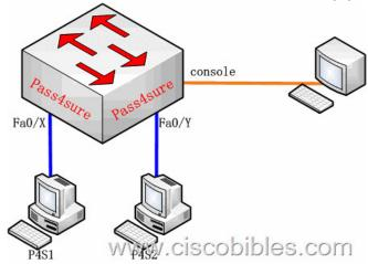
Lab Requirements: 1. Rename the switch Pass4sure. 2. The IP address of the switch is 202.103.24.86/24 and the gateway is 202.103.24.1/24. 3. The MAC address is bound. The address is 0010.7a60.1894. Lab Process: Switch>enable Switch#congfigure terminal Switch(config)#hostname Pass4sure / Rename the switch. Pass4sure(config)#interface vlan 1 / Specify an IP address for vlan1. Pass4sure(config-if)#ip address 202.103.24.86 255.255.255.05\*160; &#
