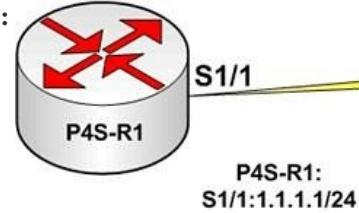
] **Lab Requirements:** Standard ACL P4S-R1 filters packets from P4S-R2. P4S-R1 configuration: 1. Create an ACL access-list 10 deny host 10.1.1.2 access-list 10 permit any 2. Apply the ACL to the interface Interface serial 1/1 Ip access-group 10 in
