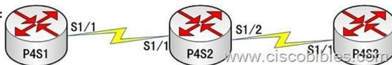
**Lab Requirements:** 1. Router name: P4S1, P4S2, P4S3 2. Set **password** to **cisco**, **secret** to **cisco1**, and **vty** to **cisco**. All the passwords are required to be encrypted. 3. Configure all these routers. **Lab Process:** Configure Router 1. Router>enable
