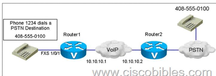
How many discrete call legs are needed to set up a call between the POTS phone attached to router 1 and the phone in the PSTN?
