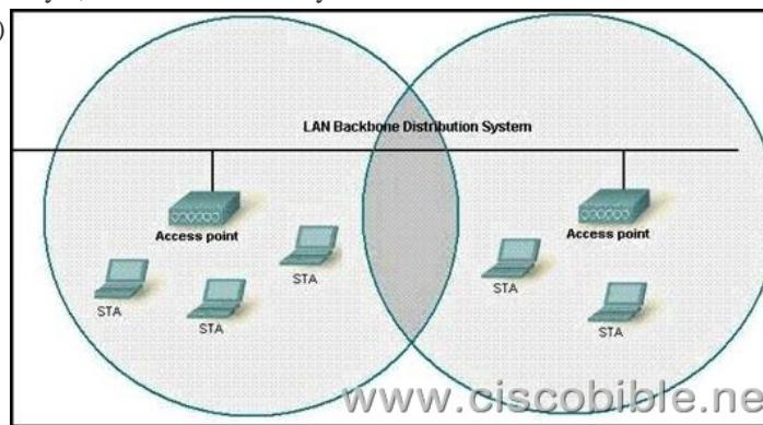
A:The area of overlap of the two cells represents a basic service set (BSS). B:The network diagram represents an extended service set (ESS). C:Access points in each cell must be configured to use channel 1. D:The area of overlap must be less than 10% of the area to ensure connectivity. E:The two APs should be configured to operate on different channels. **Correct Answers:** B, E
